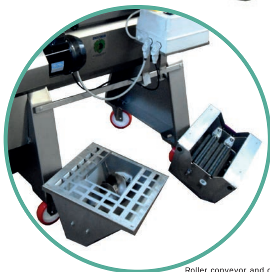
Roller conveyor and collection tank
