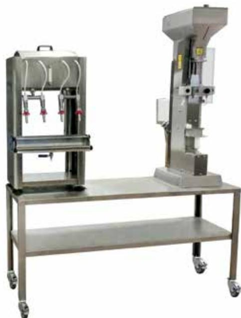
Semi-manual filling and corking monoblock adjustable according to customer needs. The system consists of an AISI 304 stainless steel desk on wheels with a length of 1400 or 2000mm; bottle filler available in both gravity and vacuum versions; corking system for cork caps (both in the pneumatic and motorized versions), screw caps, crown caps.
