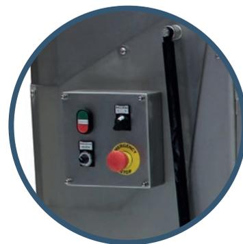
Professional destemmer with control and adjustment of the loading, destemming and crushing phases. Front opening system to facilitate disassembly and cleaning. Equipped as standard with frequency inverter, motor-gear reducer for loading hopper. Motorized crushing unit, adjustable and removable. The destemming basket is available in stainless steel or in PVC. Destemming shaft with rubber tips.
