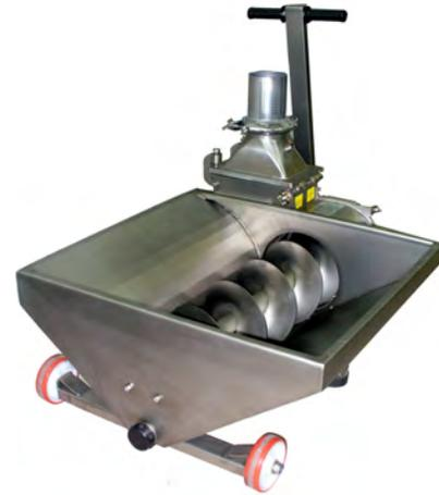
Standard fittings: opening output cone, reclining hopper and extractable control panel. If head is required or the unloading distance is considerable the installation of a compression chamber is recommended.
