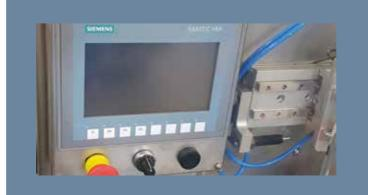
**ACCURACY:** The PLC SIEMENS allows to manage all phases of filling, adapting the machine to any type of treated liquid (wine, juice, oil, water, cream, etc. ..). The autotuning function allows the calibration of the machine automatically, eliminating the need to perform numerous samples. Repeatability volumes with an error of  $\pm$  0,5/0,2%.
