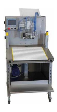
OTHER BENEFITS: large inox desk with sliding rollers and adjustable support for cardboard box; drops buffer with total drain; use of self-priming volumetric pumps with bypass and total drain valve; 7 "display; multilingual programming; oiless silenced compressor (optional).
