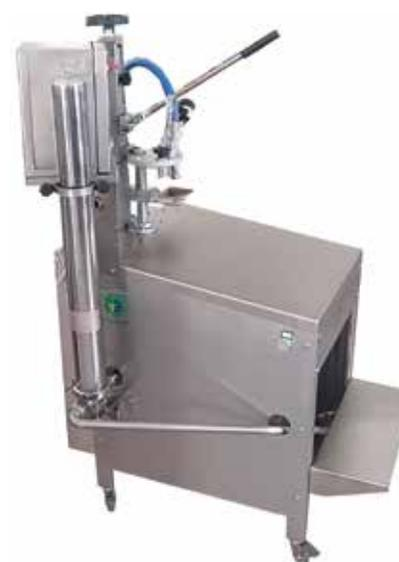
**OTHER ADVANTAGES:** use of self priming rubber impeller pump with bypass and total draining valve; filling hot liquid up to 90°C with temperature control; adjustment of filler head; inclined steel trolley; multilingual display; adjustable support for cartoon; use of pouch-up bags-cheertainer bag.
